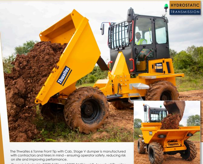
The cab is tested to ROPS 3471 and FOPS 3449 level 2. As such all Thwaites dumpers with Cab are approved for use by the UK Major Contractors Group. The Power Swivel skip enables a 90° rotation left and right, allowing the machine easier access to tip loads in restricted areas, giving the operator greater control and reducing risk on site.
