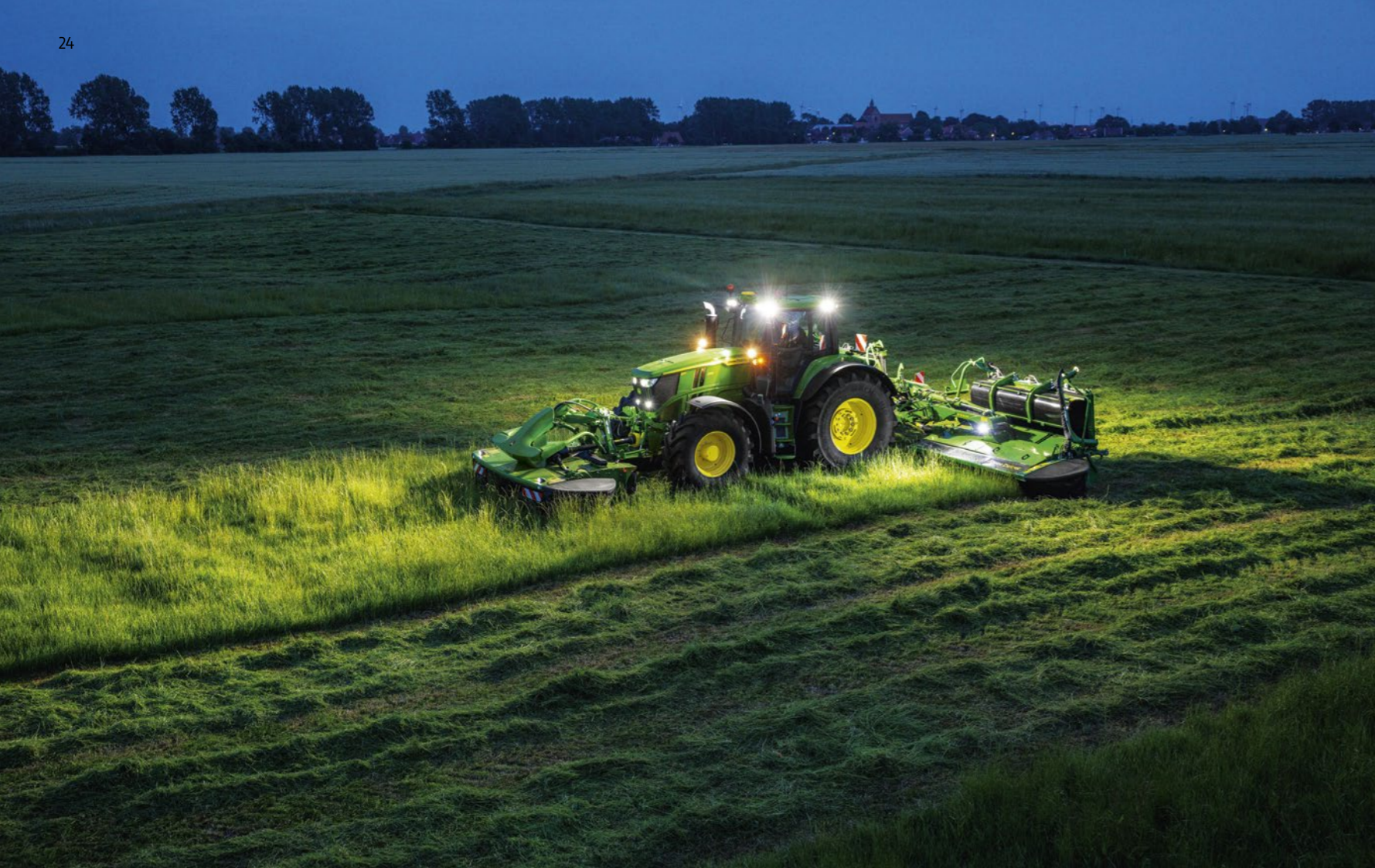
Work lights are cleverly integrated into the front, rear and sides of the roofline to prevent damage from low branches.
