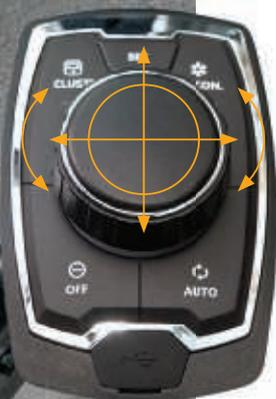
The accelerator, remote air conditioner controller and instrument cluster can be operated using the convenient jog shuttle-type **haptic controller**.
