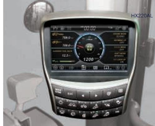
The **instrument panel** is optimised to provide quick, easy access to machine status information as you work. It features an 8-inch **touchscreen monitor** for excellent legibility.
