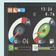
PM accumulation/ Urea accumulation display
