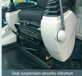
Seat suspension absorbs vibration
