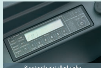
Bluetooth installed radio
