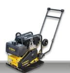
BVP 18/45 D Operating weight: 109 kg Centrifugal force: 18 kN Working width: 450 mm
