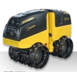
BMP 8500 Operating weight: 1,595 kg Centrifugal force: 72/36 kN Working width: 610 mm/850 mm
