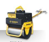
BW 71 E-2 Operating weight: 488 kg Centrifugal force: 16 kN Working width: 710 mm
