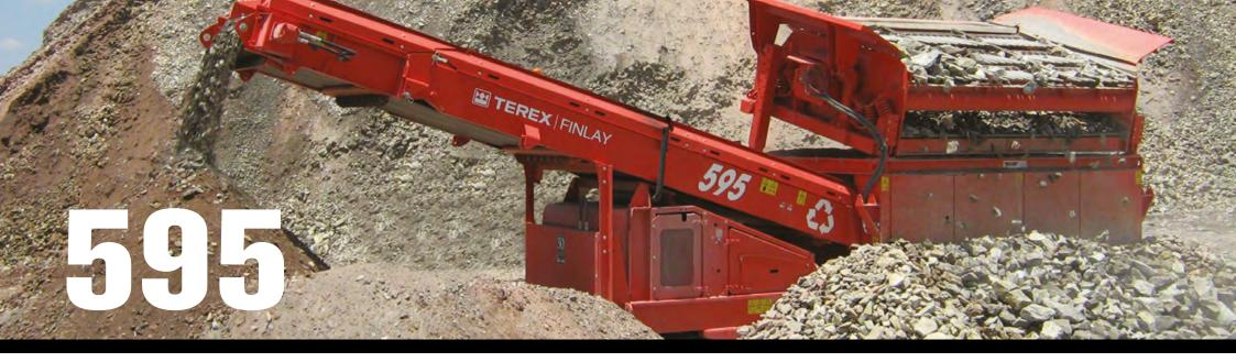
The Terex Finlay 595 Hydratrak is a self contained high capacity mobile scalping unit. Designed and constructed to the highest specification, the 595 can withstand the toughest of applications from waste reclamation projects to quarry face and demolition environments, special features include a heavy duty twin deck vibrating grid, remote control movement and a tracked undercarriage.
