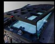
**Openable FOPS guard** The openable guard allows for easy maintenance.
