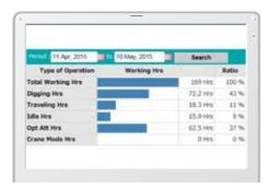
machine's operation, such as operating hours, location, fuel consumption, and maintenance status can be obtained remotely.
