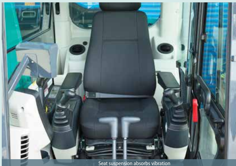
Seat suspension absorbs vibration
