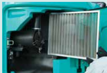
iNDr filter/radiator reservoir tank/air cleaner
